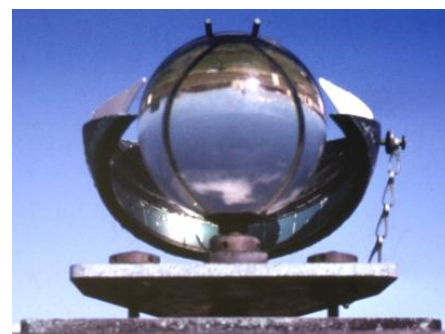
Campbell-Stokes sunshine recorder, invented by John Francis Campbell in 1853 and modified by George Gabriel Stokes in 1879. Not as common as it used to be, being replaced by modern electronic devices.
