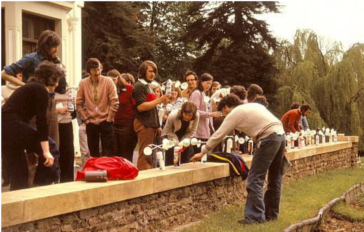
Below: Preston Montford, 1975: Alan Gadian carrying out a mass-calibration of hand-made anemometers made out of squeeze bottles and ping-pong balls. The anemometers were later deployed over nearby hills and measurements taken at pre-arranged times throughout the day. Photograph kindly supplied by Ken Bignell.
