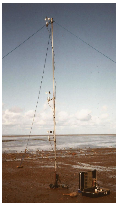
Measuring wind profiles, Blue Anchor Bay, Somerset.
